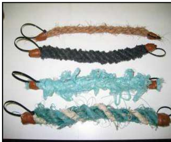
Figure 1 Rope collectors, from top to bottom: Coconut rope ( CCR ), Polipes rope ( BQR ), Christmas tree rope ( XTR ) and Galician traditional rope ( GTR )
